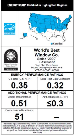
*NFRC* labels on window units give ratings for U-factor, SHGC, visible light transmittance (VT), and (optionally) air leakage (AL) and condensation resistance (CR) ratings. National Fenestration Rating Council
