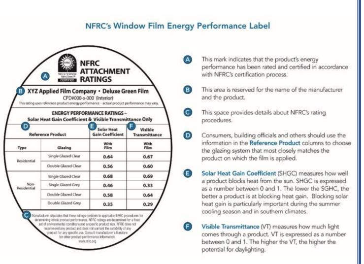
The label includes the solar heat gain coefficient (SHGC) and visible transmittance (VT) of the window film, both numbers between 0 and 1. The lower the SHGC, the better the film is at blocking heat gain. The higher the VT, the more potential for daylighting.
