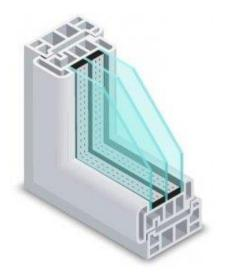
In order to minimize heat transfer between the interior and exterior of the window, the space between glazing layers, usually about 1/2", is filled with argon or krypton gas; both are inert, non-toxic, clear, and odorless.
