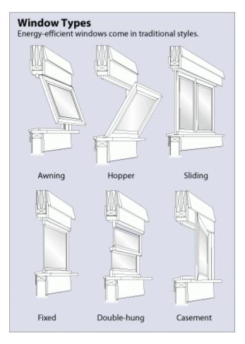
Another important consideration is how the windows operate. Since all operable windows may have undesired air leakage which will decrease your home's energy efficiency, the choice of operator type can impact overall energy use. Air leakage rates will vary with the type and quality of the weatherstripping and seals, and will generally increase over time due to operational use. Traditional operating types include:
